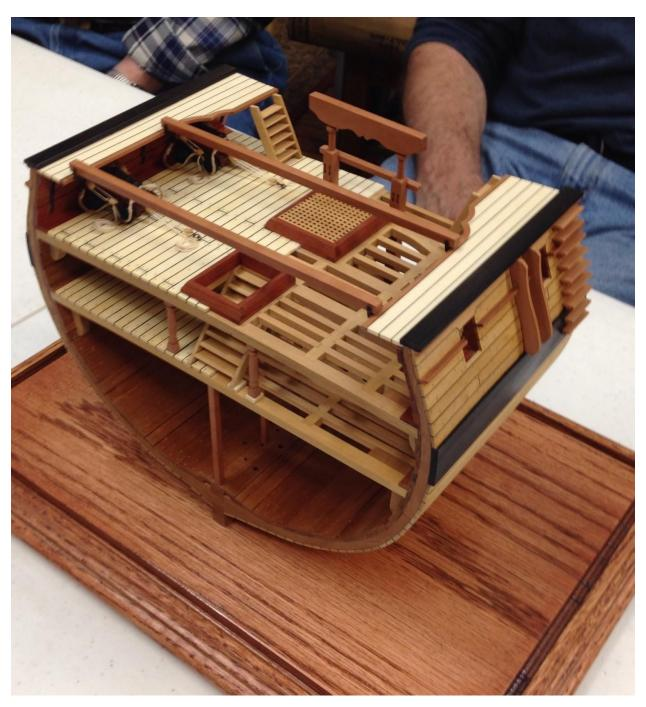
✓ Tom Lockwood: Tom settled on his work to date of the Model Expo Morgan whaler. As you can see he has completed the planking and has begun adding detail. One has to appreciate the difficulty of planking this rather small hull with what appears to be 3/16 or so bass wood. He acknowledged that the bow
