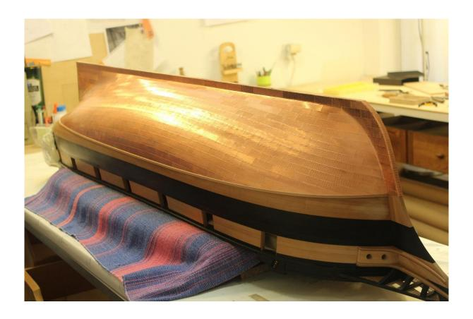
As you can see, he correctly has five rows of eleven "nails" per row. For American ships, the rows should be staggered, not in verticle lines.
